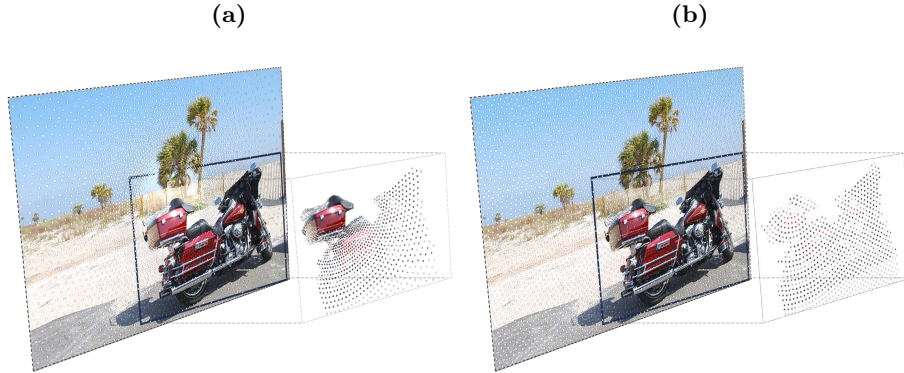
Fig. 2: Alternative sampling schemes. (a) Variable resolution with peak sample density at the center of fixation (image center in this paper) and linearly decreasing number of samples with eccentricity. (b) Uniform resolution with a constant density of samples. Both schemes distribute an equal number of samples over the entire FOV (using log-polar coordinates). In this work we address the question: which of the two alternative (motorbike) representations improves on complex visual tasks with existing DNN architectures, given that both alternatives consist of an equal number of samples?
